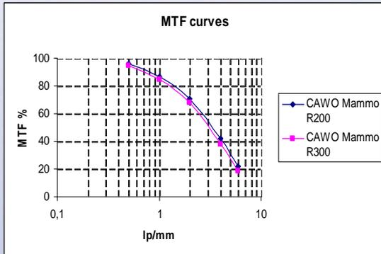
The MTF curve results from measurements which indicate a degree of the „intrinsic sharpness“ of the film-screen system as perceived on the image. The total image quality depends on other factors besides the „intrinsic sharpness“. The main factors are: graininess, noise, film, contrast, optical density and aesthetic aspects like image tint, etc.
